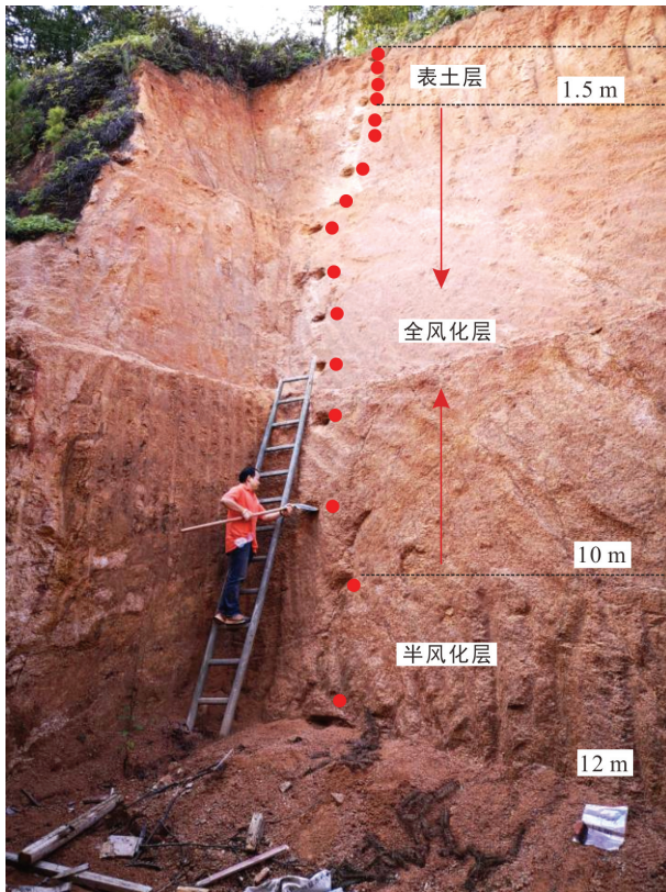
图 2 上犹岩体重稀土风化剖面及剖面采样点(红色圆点) Fig.2 The weathering profile with enrichment of HREE in the Shangyou granite batholith and sampling sites
