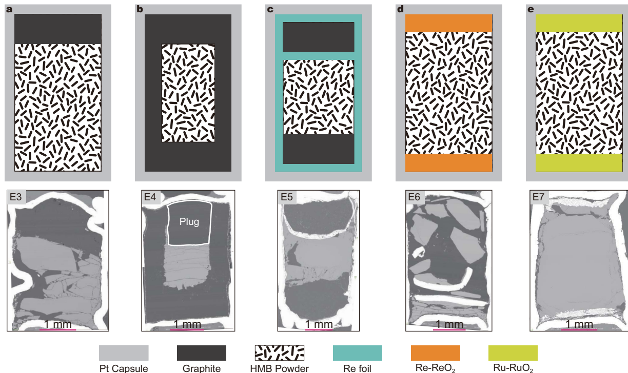
FIGURE 1. Schematic diagrams showing the sample assemblies inside the Pt capsules (the upper row), and corresponding backscattered electron (BSE) images of the experimental run products (the lower row). The experimental run number is marked in the top left of the BSE images. Note that in E6, the glass breaks into pieces during cutting and therefore it is not present in situ.
