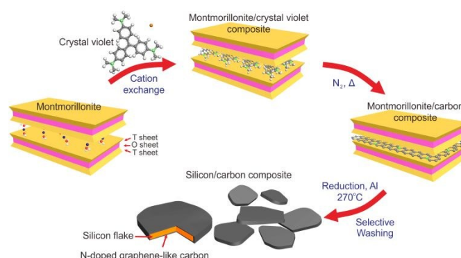
Fig. 1 Schematic illustration of the in-situ synthesis of silicon flake/nitrogen-doped graphene-like carbon composite from montmorillonite/crystal violet composite.
