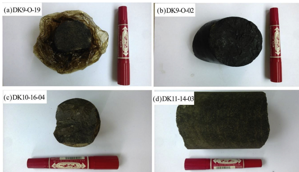
Fig. 3. Photos of drilling core samples. (a) Sandstone bearing OGI; (b) Mudstone; (c) limestone; (d) Sandstone without OGI.
