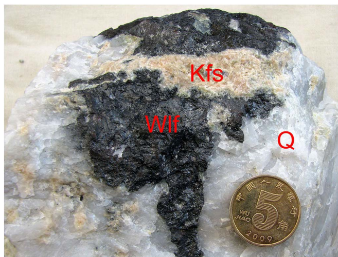
Fig. 1. Photo of a quartz-vein-type tungsten ore from Piaotang, showing post-mineralization K-feldspar veins cutting wolframite and quartz. Q: quartz; Wlf: wolframite; Kfs: K-feldspar.
