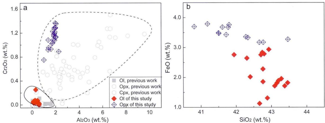
**Figure 7.** (a) Discrimination diagram for serpentine minerals formed from olivine or pyroxene. Gray-colored background data are from Dungan (1979) and Hébert et al. (1990). Serpentine that replaced pyroxene was more enriched in Al and Cr compared to that replaced olivine. (b) FeO and SiO<sub>2</sub> contents of olivine- and orthopyroxene-derived serpentine minerals in hydrated harzburgite from the Lichi Mélange, Taiwan.
