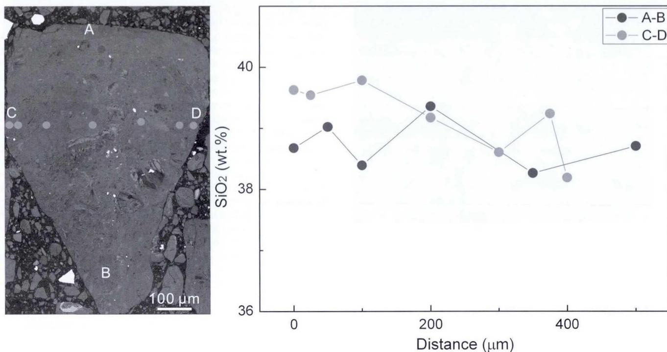
**Figure 9.** The distribution of SiO<sub>2</sub> along transects of completely serpentinized mineral fragments in the breccias, showing that SiO<sub>2</sub> is homogeneously incorporated into serpentine minerals.
