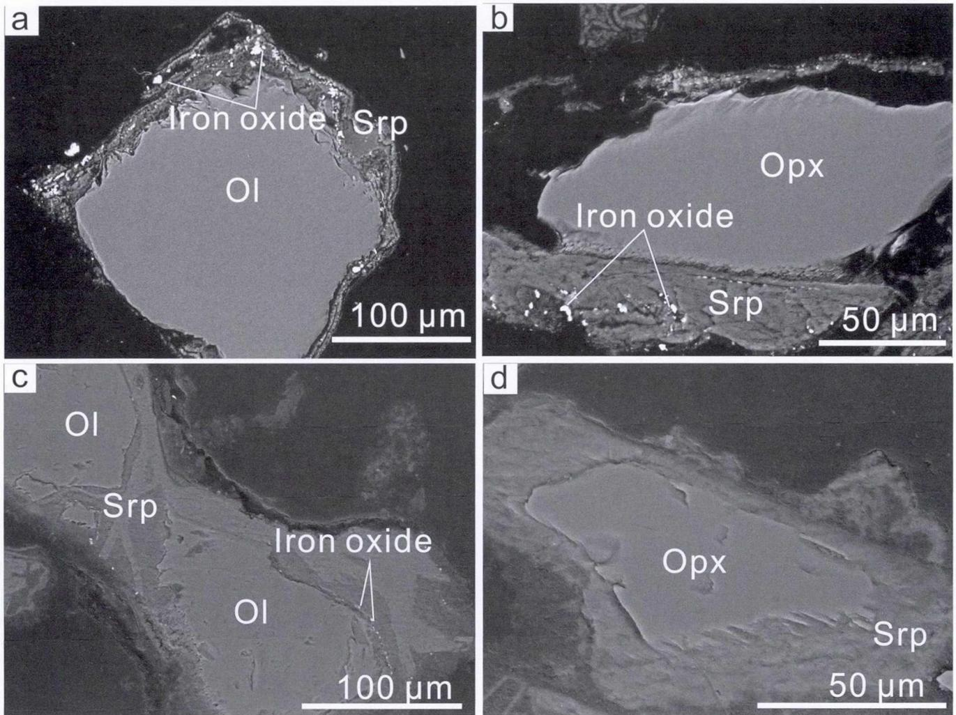
**Figure 2.** Backscattered electron images of experimental run products. (a) Fe37, olivine was replaced by serpentine and iron oxide. (b) HR42, orthopyroxene was hydrated to serpentine and iron oxide. (c) HR25, with peridotite as starting material. Olivine transformed into serpentine and a few dispersed iron oxide. (d) HR25, orthopyroxene alteration produced serpentine without forming any iron oxide.
