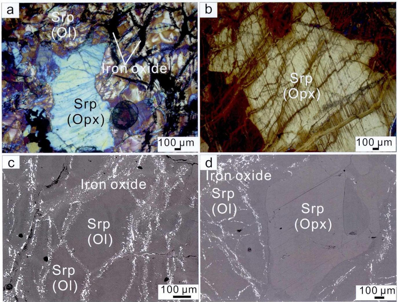
**Figure 6.** Optical and backscattered electron images of serpentinized harzburgite from the Lichi Mélange, Taiwan. It shows that all iron oxide was distributed around olivine pseudomorphs, and it was absent around orthopyroxene pseudomorphs. Srp (Ol), olivine-derived serpentine; Srp (Opx), orthopyroxene-derived serpentine.
