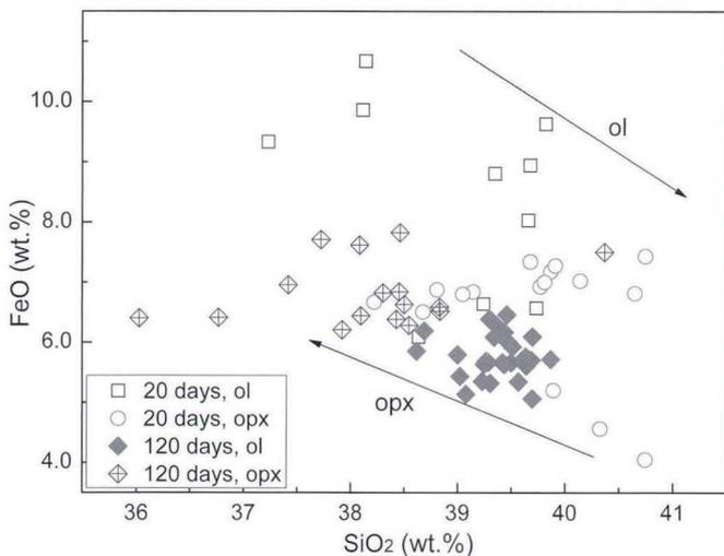
**Figure 5.** Silica and FeO contents (wt.%) of serpentine minerals formed from olivine and orthopyroxene. ol—olivine; opx—orthopyroxene.
