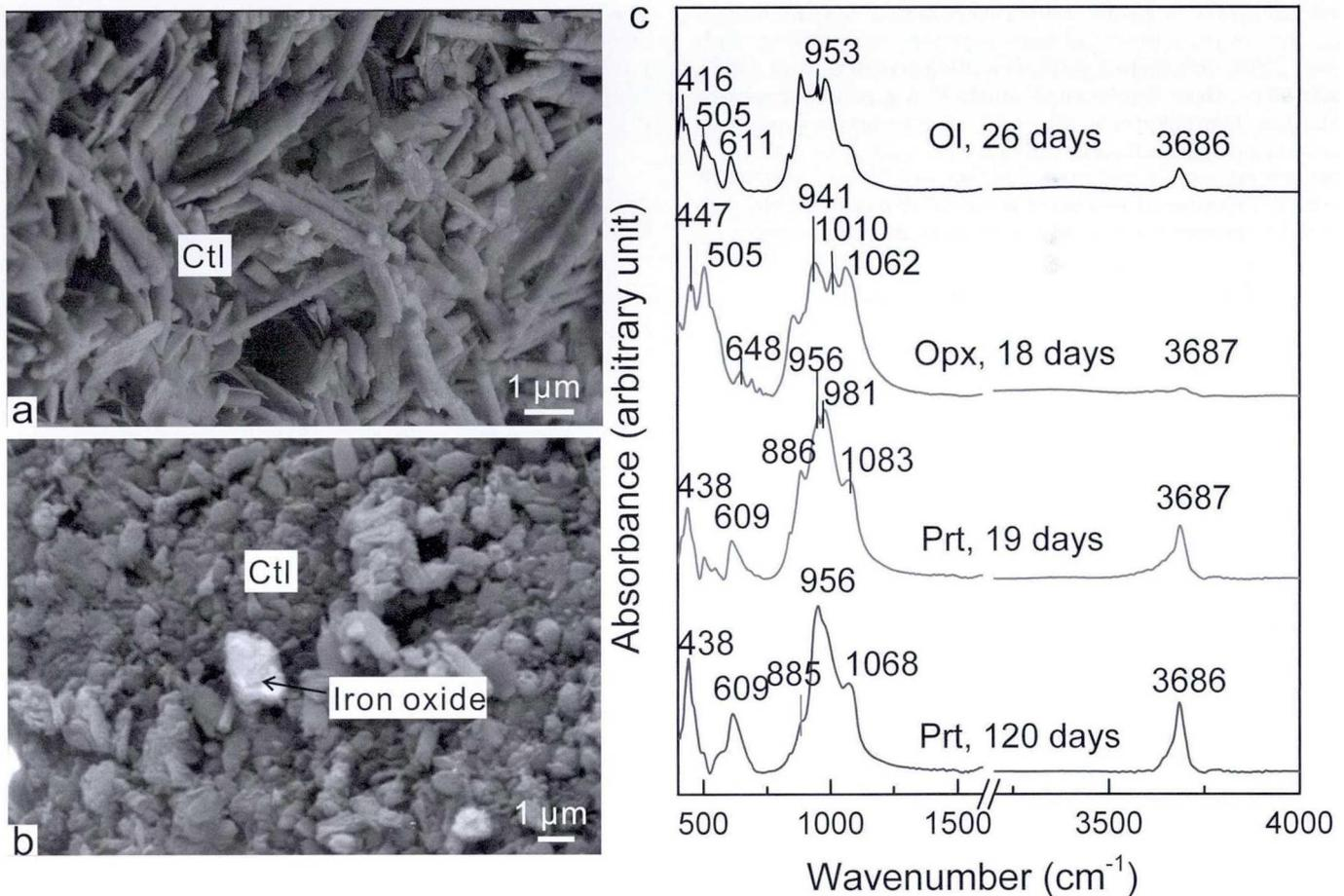
**Figure 1.** Identification of solid products based on scanning electron microscope images and Fourier transform infrared spectra. (a) HR61, with peridotite as starting material. Fibrous chrysotile was formed. (b) Fe37, with olivine as starting material. Fibrous chrysotile and iron oxide were produced. (c) Infrared spectra of solid products, showing that serpentine was the main secondary hydrous mineral.
