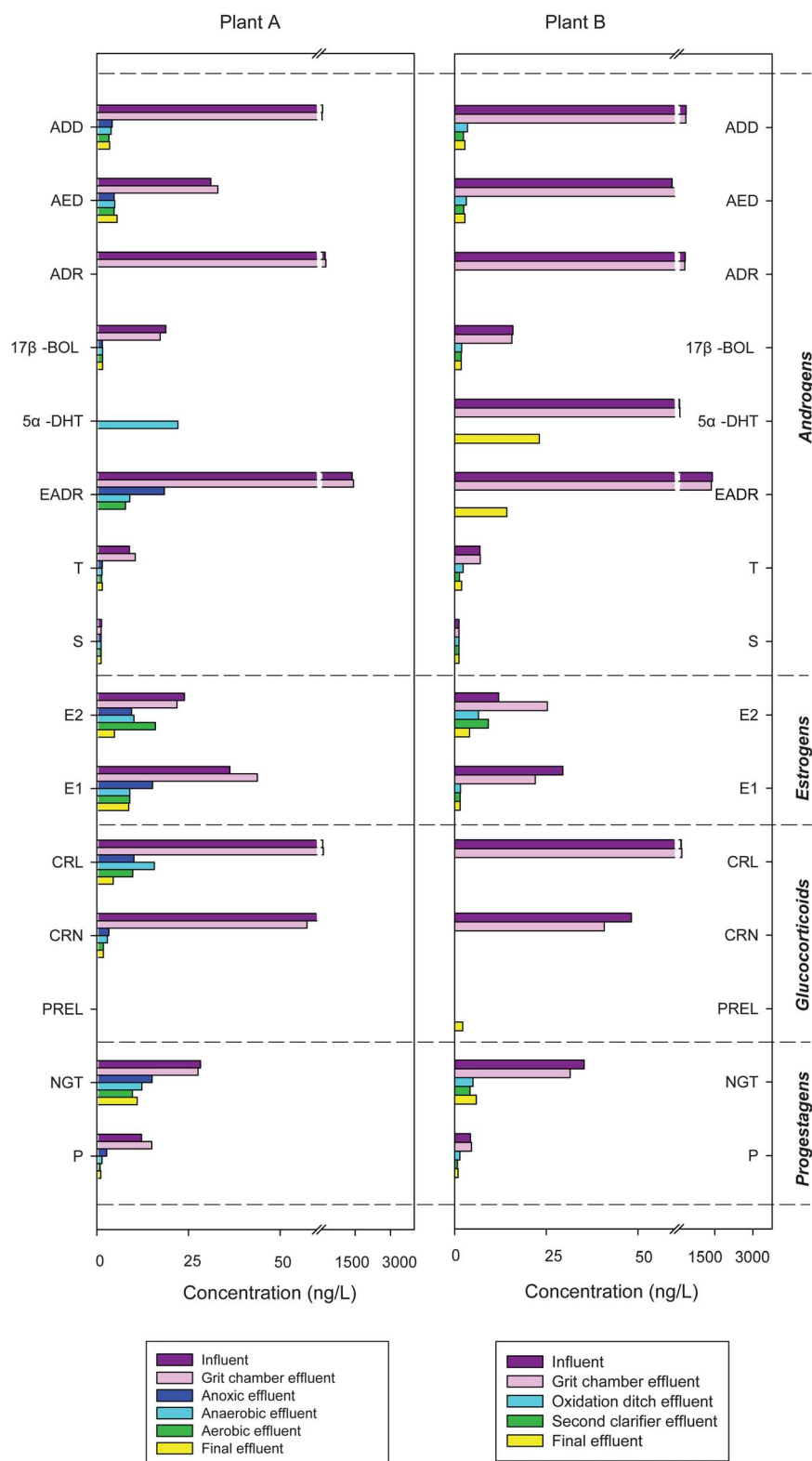
Fig. 2 Concentrations ( \text{ng L}^{-1} ) of androgens, estrogens, glucocorticoids and progestagens in influent, grit chamber effluent, anoxic effluent, anaerobic effluent, aerobic effluent and final effluent of Plant A and Plant B. For compound abbreviations, please see Table 1.
