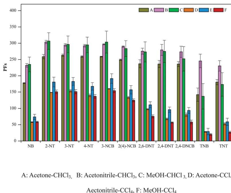
**Fig. 1** Pre-concentration factor of the NBs and NCBs; samples spiked to 5.0  $\mu\text{g L}^{-1}$  of each analyte. Extraction conditions: aqueous sample volume 5.0 mL; extraction time: 2 min; sedimented phase controlled to  $10.0 \pm 0.5 \mu\text{L}$ .
