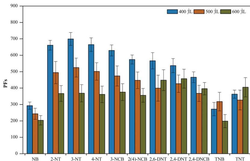
**Fig. 3** Effect of the volume of the dispersion solvent (acetonitrile) on the PFs of the NBs and NCBs. Extraction conditions: sample volume, 5.0 mL; extraction solvent, 40.0  $\mu\text{L}$   $\text{CHCl}_3$ .
