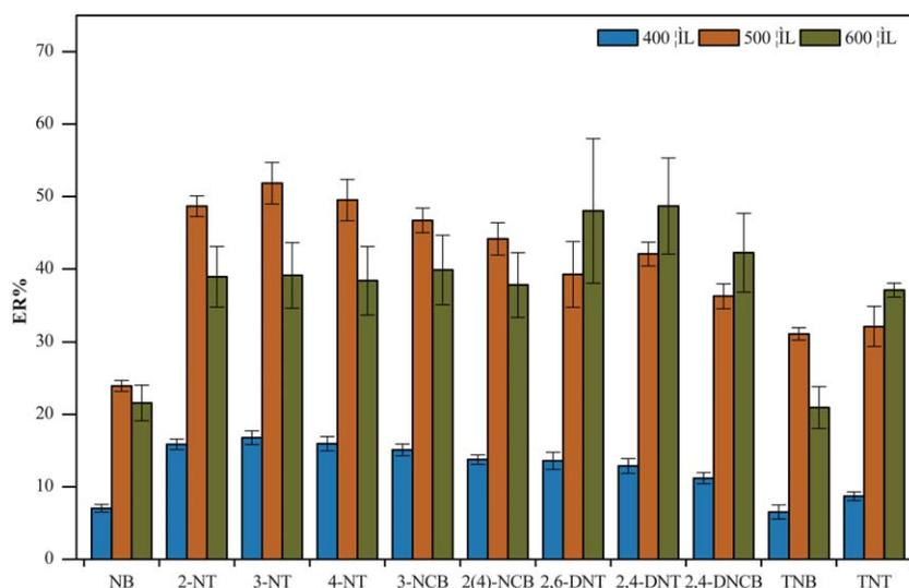
**Fig. 4** Effect of the volume of the dispersive solvent (acetonitrile) on the ERs of the NBs and NCBs. Extraction conditions: sample volume, 5.0 mL; extraction solvent, 40.0  $\mu\text{L}$   $\text{CHCl}_3$ .
