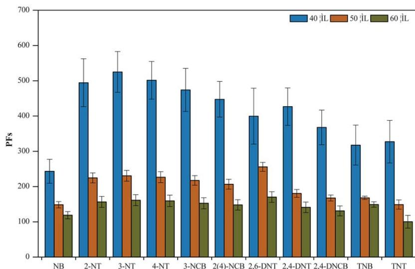
**Fig. 2** Effect of the volume of the extraction solvent ( $\text{CHCl}_3$ ) on PFs of the NBs and NCBs. Extraction conditions: sample volume: 5.0 mL; dispersion solvent: 500.0  $\mu\text{L}$  acetonitrile.
