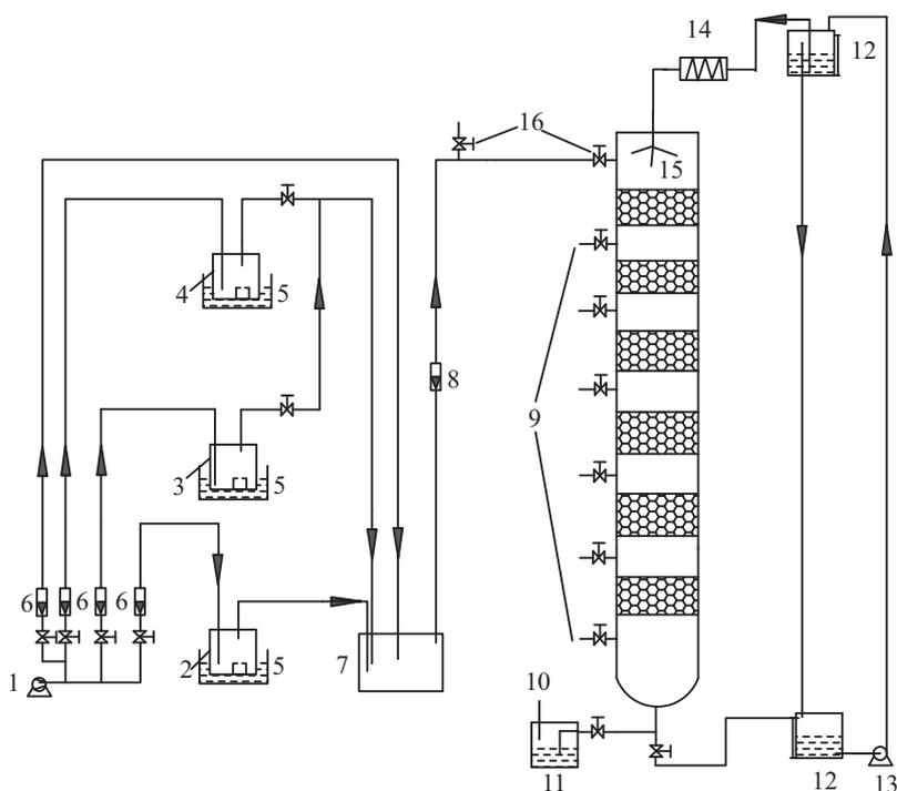
**Fig. 1.** Schematic diagram of the biotrickling filter: (1) air pump; (2–4) VOSCs reservoir; (5) water bath; (6 and 8) mass-flow controller; (7) mixing gas tank; (9) gas sampling and pressure determination ports; (10) gas out; (11) exhaust gas recycling bottles; (12) nutrient recirculation tank; (13) mass-flow pump; (14) peristaltic pump; (15) nutrient distributor; (16) valves.
