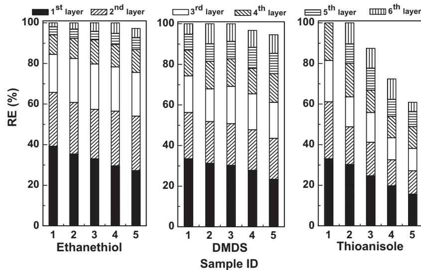
**Fig. 4.** REs of ternary mixture of ethanethiol, DMDS and thioanisole at different ratios (ethanethiol:DMDS:thioanisole = E:D:T): (1) E:D:T = 6:4:1; (2) E:D:T = 3:2:1; (3) E:D:T = 6:4:3; (4) E:D:T = 3:2:2; (5) E:D:T = 6:4:5.
