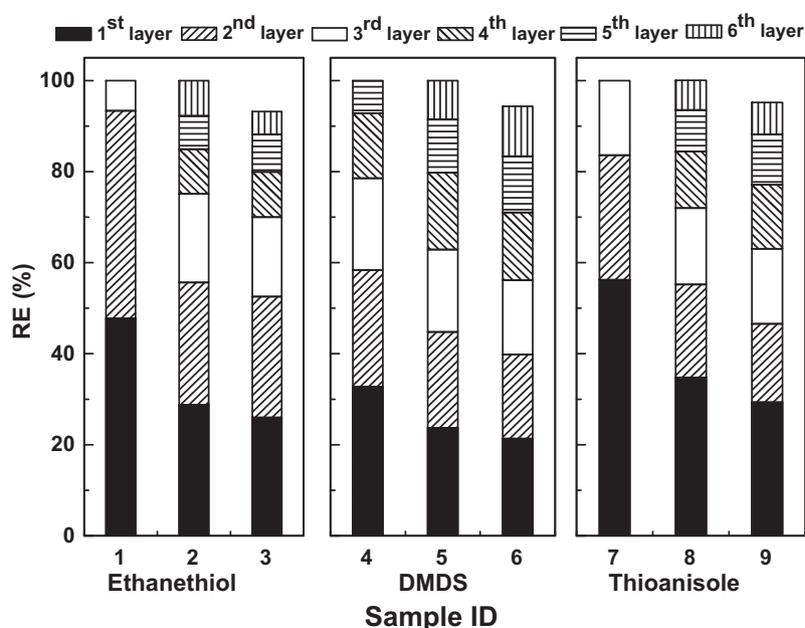
**Fig. 2.** REs of ethanethiol, DMDS and thioanisole as a single substrate at different inlet concentrations (mg/L): (1) 0.42; (2) 1.05; (3) 1.21; (4) 0.29; (5) 0.81; (6) 1.04; (7) 0.13; (8) 0.33; (9) 0.41.
