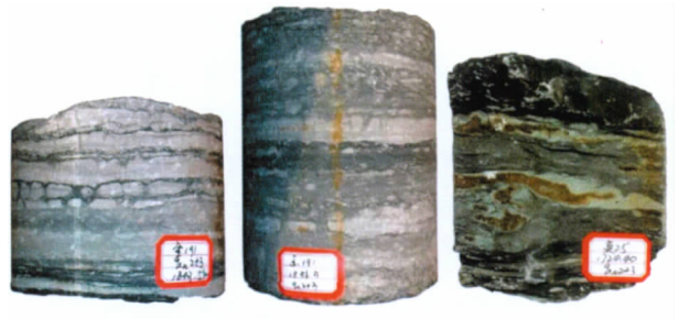
图 8 肠状、串珠状、蠕虫状砂脉岩心照片 Fig. 8 Core photo showing ptigmatic, beaded and verm-like sand vein
