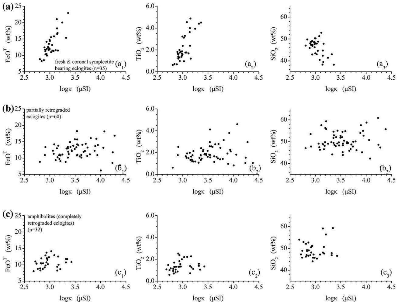
**Fig. 5.** Major oxides  $\text{FeO}^T$ ,  $\text{TiO}_2$  and  $\text{SiO}_2$  versus logarithmic bulk magnetic susceptibility ( $\log \kappa$ ) of eclogites from the CCSD main hole: (a) fresh & coronal symplectite-bearing eclogites, 35 samples; (b) partially retrograded eclogites, 60 samples; (c) amphibolites (completely retrograded eclogites), 32 samples.
