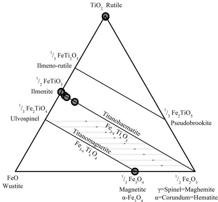
**Fig. 6.** Ternary FeO–Fe<sub>2</sub>O<sub>3</sub>–TiO<sub>2</sub> diagram showing compositions of Fe–Ti oxide minerals in eclogites from the CCSD main hole.
