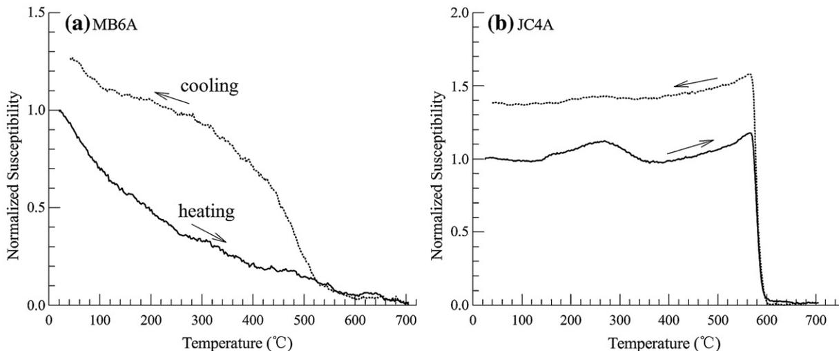
Fig. 4. Normalized thermomagnetic curves in argon, calibrated against an empty furnace: (a) fresh eclogite MB6A; (b) strongly retrograded eclogite JC4A. Heating curves, solid lines; cooling curves, dashed.
