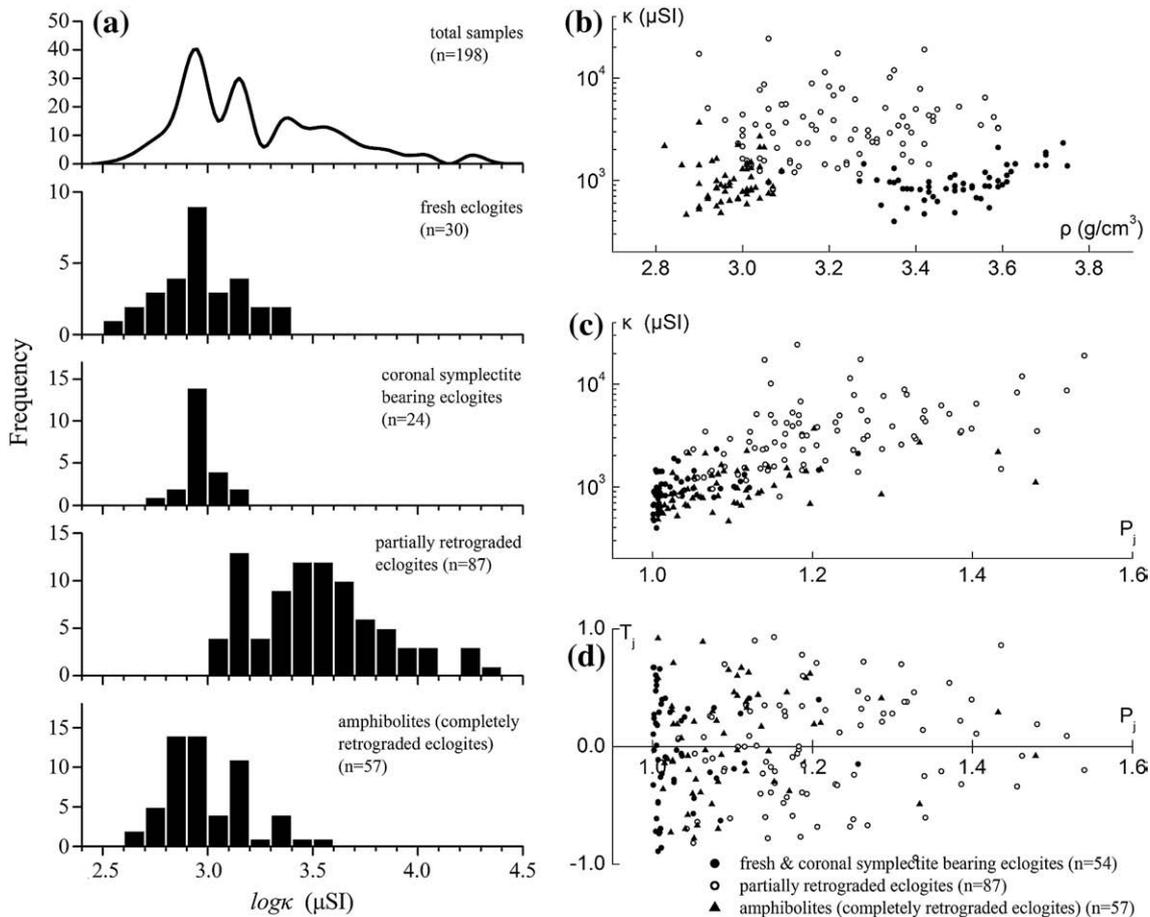
Fig. 3. Low field AMS values of eclogites from the CCSD main hole and surface outcrops in the Donghai area, southern part of the Sulu UHP metamorphic belt. (a) Frequency distributions of logarithmic magnetic susceptibility  $\log\kappa$  from variably retrograded eclogites. (b) Bulk magnetic susceptibility  $\kappa$  versus density  $\rho$ . (c) Corrected anisotropy degree  $P_j$  versus  $\kappa$ . (d) Shape parameter  $T_j$  versus  $P_j$ .
