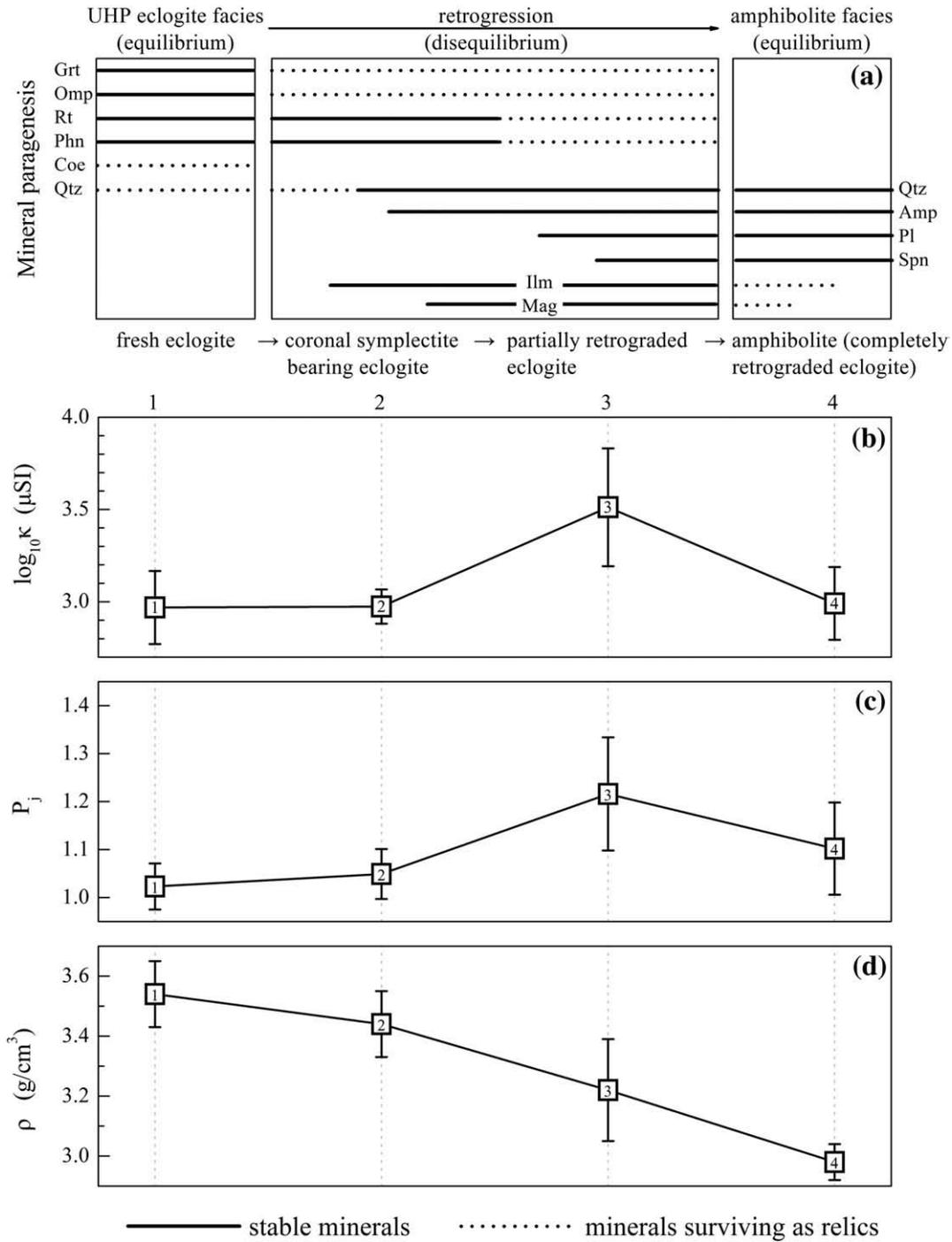
**Fig. 7.** (a) Summary of retrograde metamorphic evolution of minerals in eclogites; (b) evolution of logarithmic bulk magnetic susceptibility  $\log \kappa$ ; (c) corrected anisotropy  $P_j$ ; (d) bulk density  $\rho$ ; b,c,d, time scale as in a. Samples as in Fig. 3, error bars 1 SD.
