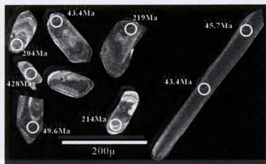
图2 样品 D5144-1 代表性锆石阴极发光图像 Fig. 2 Cathodoluminescence image of representative zircons from sample D5144-1
