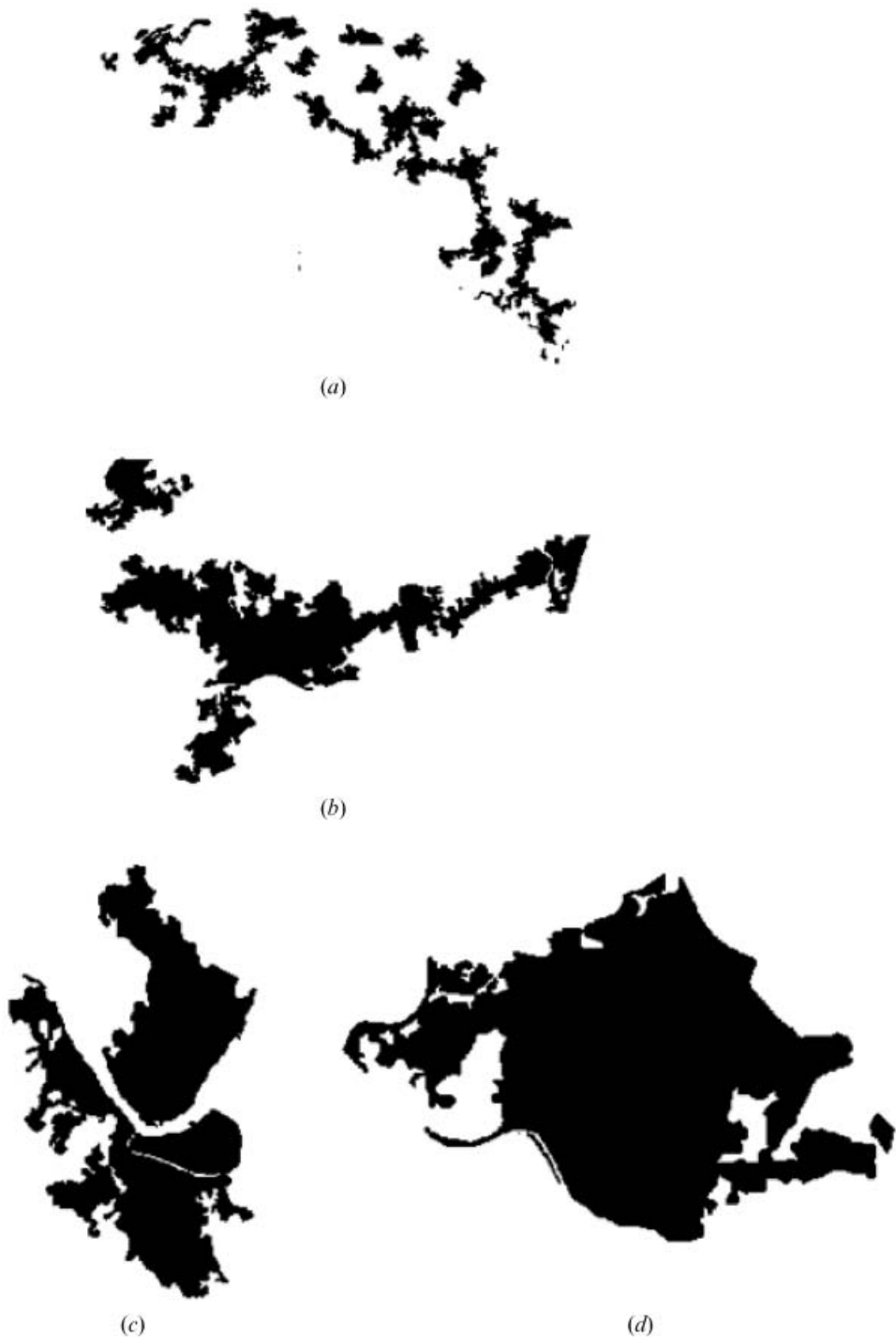
Figure 6. Four typical urban forms with different urban compactness values. (a) D=1.67 ; (b) D=1.77 ; (c) D=1.88 ; (d) D=1.96 .
