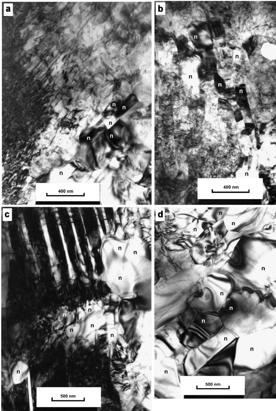
Fig. 7. TEM (bright field) micrographs showing typical substructures of dislocations and dynamic recrystallization in anorthite deformed by torsion at P=400 MPa, T=1473 K, \dot{\theta}=3.0 \times 10^{-4} rad/s. The distribution of dislocations is heterogeneous and grain boundary migration toward highly strained grains with very high (tangled) dislocation density forms recrystallized grains ( n ). (a), (b) and (d) from a pure anorthite aggregate; (c) from an anorthite layer in a layered Qtz–An sample; (d) from a C' shear zone.
